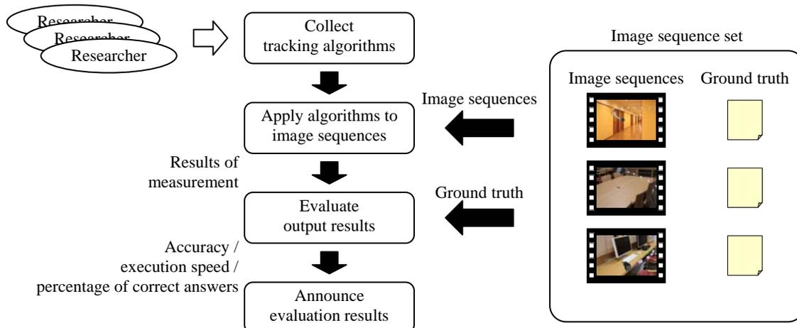
Figure 1. The process of evaluation at the 1st phase.
